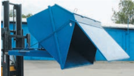
Easy and safe control from the driver's seat. Self-acting cover opening.
