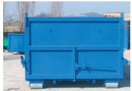
Flap, hinges on top + screws.
